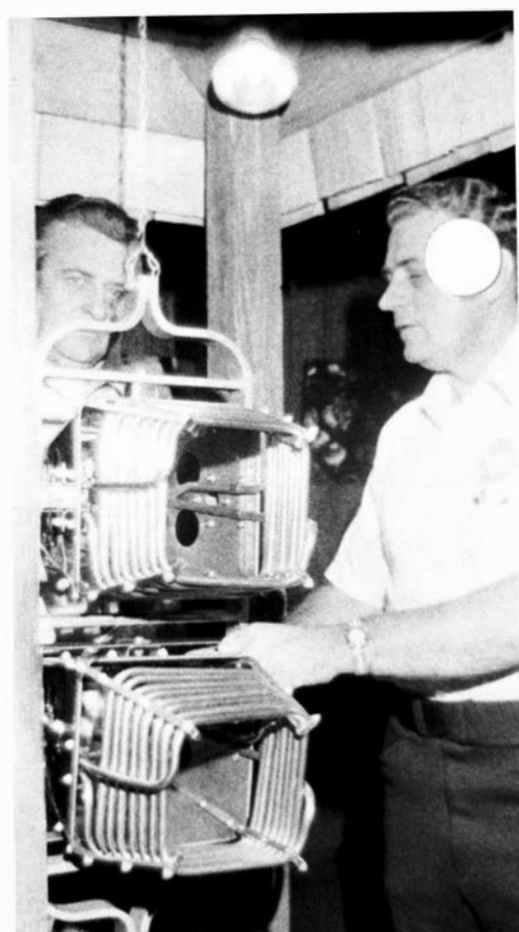
GADO inspectors Harold Phillips (left) of Lubbock, Tex., and Travis Boren of Houston inspect a propane burner during the Albuquerque seminar on balloon certification and inspection.
