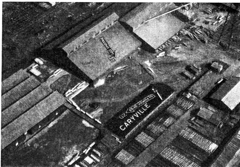
FIGURE 5.—The above picture shows how a group of buildings may be utilized in order to obtain larger lettering than would be possible on a single roof. Note that the marker placed on a light-colored roof in the upper center of the picture has been outlined in black to provide sufficient contrast, whereas this is not necessary on the dark-colored roof.
