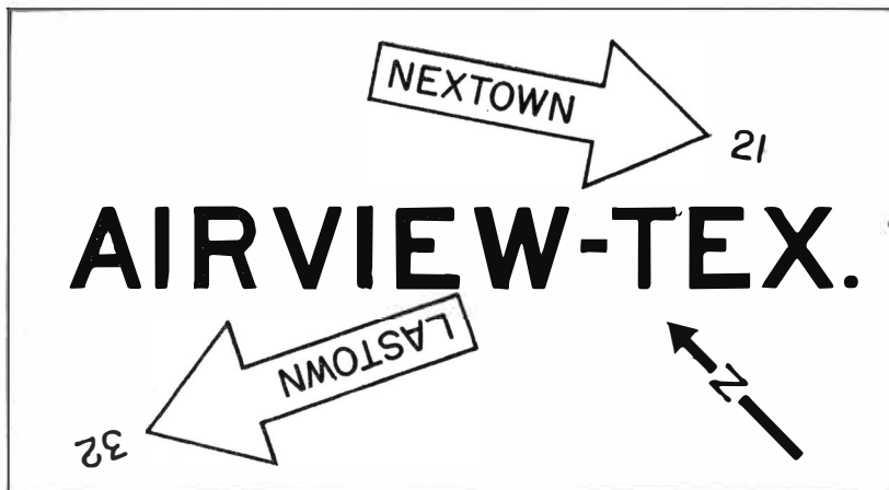
FIGURE 2.—Intermediate town marker. This marker includes the name of the town and State, the meridian marker, and shows direction and distance to nearby towns having airports.
