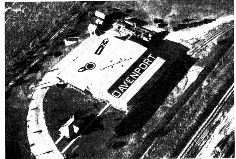
FIGURE 8.—Air marker painted on light-colored roof. Note selection of prominent roof adjacent to highway and railroad. Also note old air marker on top section of roof and the contrast of its effectiveness with the new standard marker. To complete the air marker the abbreviation for the name of the State should be added.
