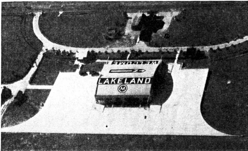
FIGURE 22.—Air marker on a hangar roof. In the case of a municipal airport the letter M, enclosed in a circle to prevent confusion in reading the sign, may be used instead of repeating the name of the city. The abbreviation for the name of the State should be added to complete the sign.
