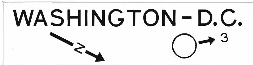
FIGURE 1.—Typical airport town marker includes the name of the city and abbreviated name of State, meridian marker with arrow pointed true north, and circle airport symbol with arrow and numeral indicating the direction and number of miles to the airport.
