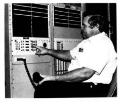
Working on integrated communications switching system equipment at DeRidder's Automated Flight Service Station is electronics technician Bill Kenney.
