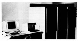
The workhorse of RMM is the Maintenance Processor Subsystem—the computer that queries the facility, processes its data, stores it and takes remedial instructions back to the facility.
