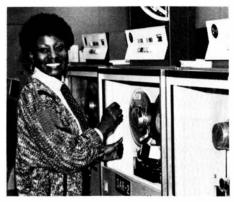
Computer operator Beverly Faber changes a system analysis recording tape on the center's IBM 9020 computer.
