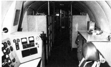
The flight inspection work station and avionics equipment racks looking aft.
