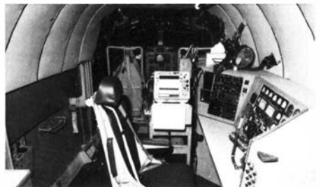
The flight inspection technician checks navigation aids parameters at his console and on the recorder to his left.
