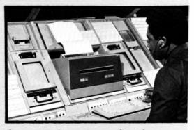
Computer update equipment (CUE) for flight data processing, shown here at the Memphis ARTCC, includes complete alphanumeric keyboard, flight strip printer and visual computer readout devices (on each side of the printer).
