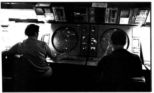
Primary and beacon radar required the use of shrimp boats to keep track of aircraft, as shown at the Kansas City Center around 1969 (top). With the advent of computerassisted radar, alphanumeric data tags were placed right on the scope, shown here at the Washington ARTCC in 1983 (above).
