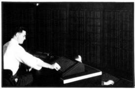
One of the earliest attempts at automating ATC functions was this Teleregister Flight Progress Board at the Washington Airway Traffic Control Center in 1941. Airline radio operators would transmit flight information to the center, where flights could be rapidly resequenced. The board also provided collision alerts.
