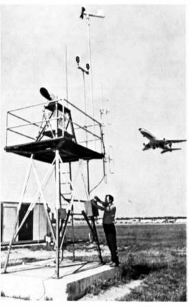
Electronics technician Wilbur Horton checks one of the earliest LLWAS sensors in a test at Atlanta International Airport. This boundary remote unit has the Fairchild configuration.
