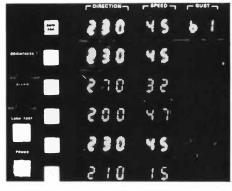
The local controller display in the tower cab continuously indicates wind direction, speed and gusts and sounds an alarm and flashes when wind shear of 15 knots or more occur. Photo courtesy of Fairchild Weston Systems
