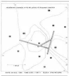
radio or telephone lines to a computer, which compares the sensor readings and analyzes the information. If any of the sensors shows a variation in wind exceeding 15 knots, except for gusts, the system provides a warning to tower controllers.
