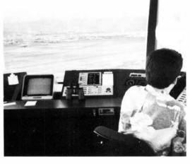
One of the local controller displays in the Honolulu Tower provides the controller with a LED display of wind speed and direction for each sensor and an aural alarm if wind variation exceeds 15 knots.
