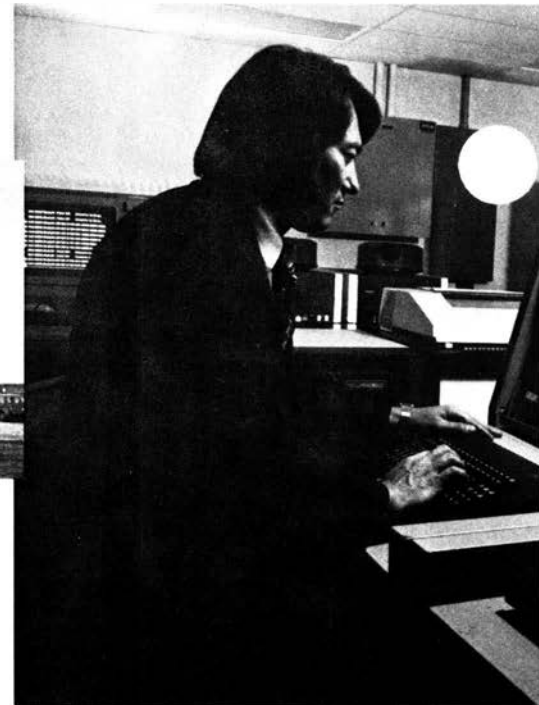
At the Cleveland ARTCC, George Krell, an E-Systems engineer providing contract support for FAA, operates the computer operator terminal console, which can monitor and interact with all the automated stations in the family.
