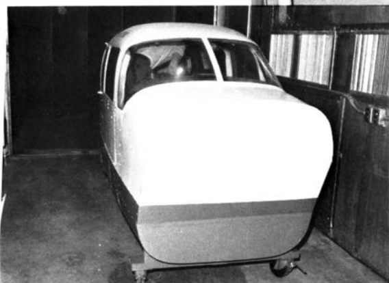
With the temperature at 25 degrees below zero and falling in a CAMI ice box cum wind tunnel, an FAA pilot seeks his survival gear inside a simulator.
