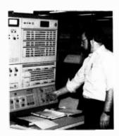
Computer technician Robert Hirsch prepares to load a diagnostic program into the center's IBM 9020 computer.
