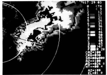
moving, separated "hard" targets like aircraft, it is less successful with randomly distributed masses of moisture-laden particles suspended in the air, which have a velocity spectrum wholly beyond its capability to measure.
