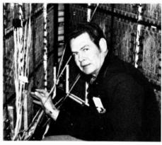
Bob Hutchins, central computer complex technician in the Flight Data Processing Unit, attaches logic analyzer pobes to the compute element 1 of the IBM 9020A.
