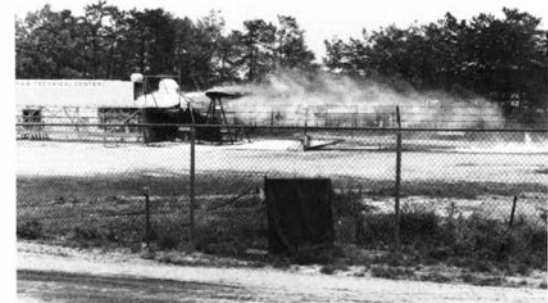
Much experimentation went on at the Technical Center's wing spillage facility to judge the potential of the antimisting kerosene fuel additive. These photos show the effects of igniting conventional fuel (top) and treated fuel (above) in an induced wind over the wing surface.
