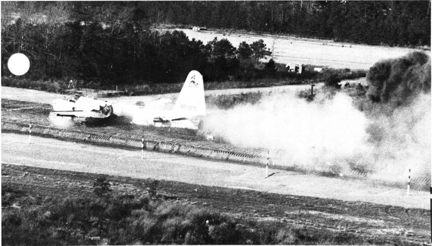
Closer to the reality of the current controlled-impact demonstration were the tests conducted at the Lakehurst, N.J., Naval Air Engineering Center in which whole aircraft were rocket driven along the ground into obstructions to rupture the fuel tanks. The fireball (left) resulted from untreated fuel; virtually no fire resulted from treated fuel (above).
