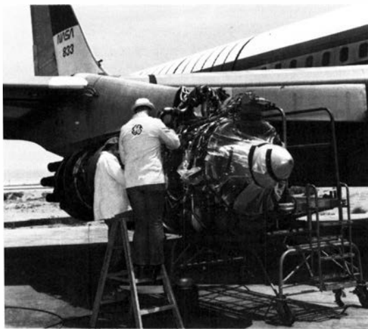
General Electric mechanics adjust the degraders in the aircraft's engines, which restore the fuel to a burnable state.
