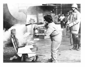
With a fireman in readiness as an extra measure of safety, a Tech Center employee uses a carbon dioxide extinguisher on an airline seat fire.
