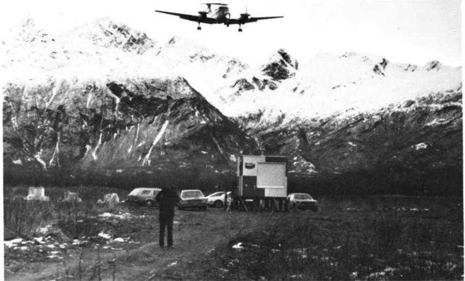
The first microwave landing system commissioned in the country was at Valdez, Alaska, in November 1982. MLS provides a cleaner signal, as well as the potential for multiple glide slope angles and segmented and curved approaches.
