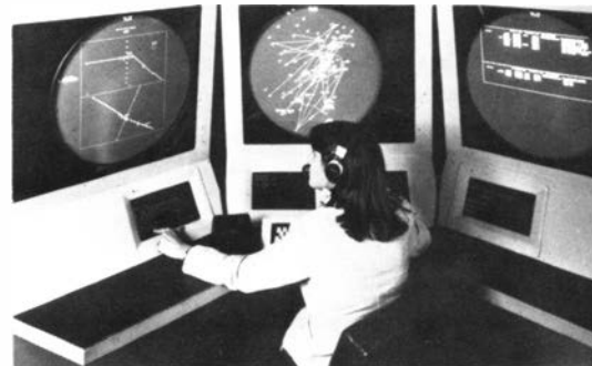
The controller's sector suite of tomorrow being tested at the Mitre Corp. At left is the "planning display"; at right is flight data; at center is the usual plan view display. All are shown with touch entry.
