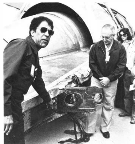
Elwood Driver (left), then vice chairman of the NTSB, points to a faulty engine pylon forward support from the DC-10 that crashed in Chicago in May 1979.
