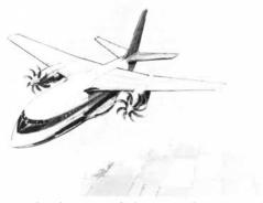
The thinner and shorter eight- to 10-blade, swept-tip propeller, or propfan, is expected to offer quieter, fuel-efficient operation at speeds comparable to those of jetliners.
