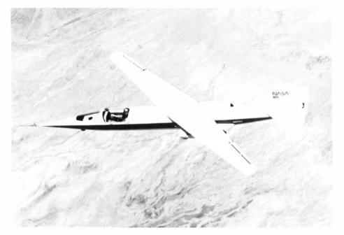
Rutan built this oblique wing (skew wing, scissors wing, swing wing) for testing at NASA's Dryden Flight Research Center. Called the AD-1 (Ames/Dryden), the research vehicle has a wing that can pivot up to 60 degrees from perpendicular to the fuselage and is proving its projected stability, quieter takeoffs, higher speed and reduced-fuel capabilities. It's believed that a future oblique-wing transport could fly at 1,000 mph at twice the fuel economy of conventional SSTs.
