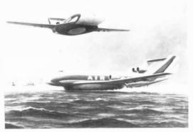
One NASA answer to the constraints of airport size and the need for larger cargo aircraft is the air-cushion landing gear irfreighter, which could use runways, water and even unprepared sites. Bell Aerospace Textron has studied it.
