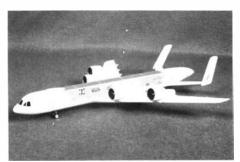
Another approach to handling air cargo is Lockheed-Georgia's concept of a flatbed aircraft that could handle containerized cargo as shown, outsized equipment like a construction crane or even passengers in an add-on module.
