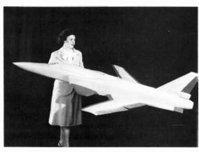
Langley aerospace engineer Sue Grafton holds a wind-tunnel model of a Grumman forward-swept-wing aircraft. This configuration permits the wingtips to remain unstalled at high angles of attack.
