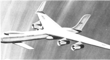
his configuration is for a global-range nuclear-powered argoliner for payloads of 200 tons. It would use supercritical airfoils, a free-floating canard with spanwise blowing for horizontal control and high-bypass-ratio engines.
