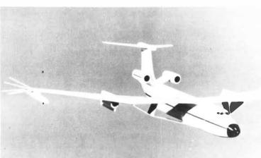
This NASA Langley Research Center Model reflects a commuter version of a natural laminar flow control aircraft with pusher propfans. The aircraft would use a high-aspect-ratio wing, and both fuselage and wings would be clear of any flow-disrupting sufaces. (top)
