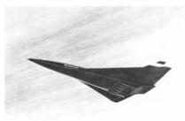
A dual propulsion hypersonic airliner has been studied by Lockheed-California for NASA. The liquid-hydrogen-fueled aircraft would use five conventional turbojets as boosters for five supersonic combustion ramjets to move it at 4,000 mph at 110,000 to 120,000 feet. Its range would be over 5,400 miles.
