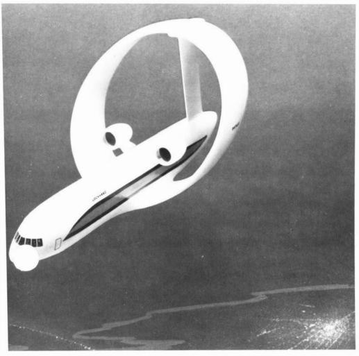
The Ring Wing of the Lockheed-Georgia Co. is a design for the next century. It's thought to offer lower drag and half the wing weight for the same payload capacity. Wind tunnel tests are underway.
