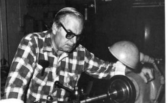
Machining a shaft for a gear box that will operate hangar doors at the Flight Operations Building is Albert Colwell.
