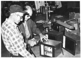
Norman King (left) and William Mayer work on displays to modify TRACON consoles for the center's simulation lab.
