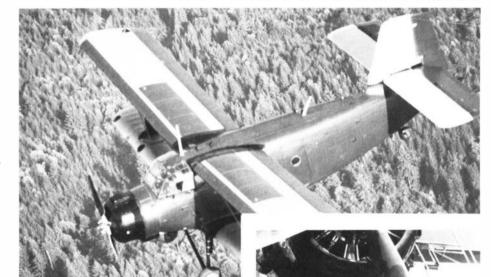
aluminum, it's 7,276 pounds empty and over 11,000 pounds at gross, holding two in the cockpit and 14 passenger seats. It cruises at 124 mph; top speed is 161; its range 560 miles; and its ceiling 16,400 feet. It has a Shetsov air-cooled radial engine that develops 1,000 hp, driving a four-blade, variable-pitch, constant-speed propeller.
