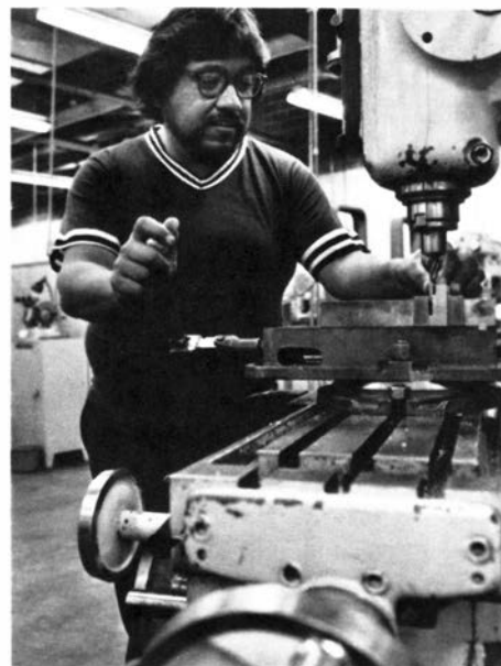
Machinist Leonard Maldonado makes an obsolete air gap gauge for a rotary coupler for the Trinidad, Colo., ARSR-2.
