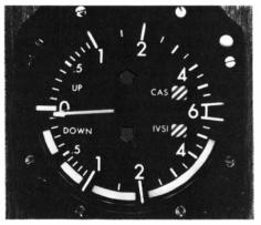
Another display to be found in a TCAS IIequipped plane is a modified instantaneous vertical speed indicator (IVSI), here indicating the resolution advisory "do not descend" by means of the lighted bars. The pilot must keep the IVSI pointer out of the descent rates covered by the illuminated segments. An alternate climb or descend advisory could be displayed by lighting the appropriate arrow in the center of the instrument.
