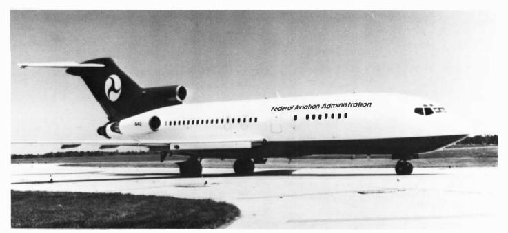
This FAA B-727 will be a test bed for TCAS II engineering prototypes.
