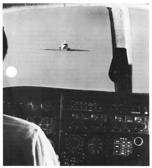
Two FAA Technical Center aircraft—a B-727 and a Convair 580—really fly at each other deliberately to trigger collisionavoidance equipment installed in their ockpit panels.
