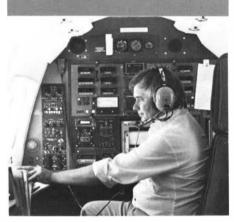
Electronics technician Don Stokes' office during a flight check is a compact, computerized array of avionics at the rear of a Sabreliner flight-inspection plane.
