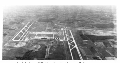
Aerial view of Dulles showing its parallel runways. The aircraft parking and service area is the horizontal light-colored strip beyond the tower and terminal.
