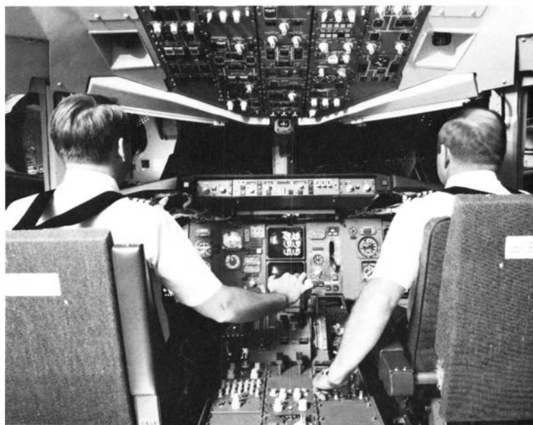
Eastern Air Lines acceptance pilots fly a Phase II simulator for a Boeing 757.
