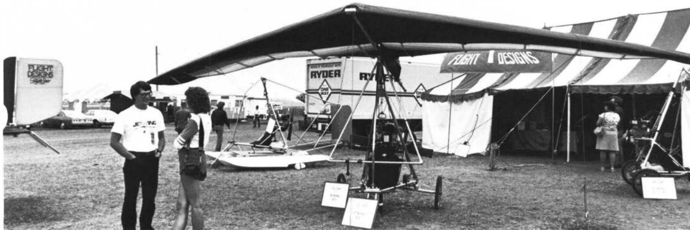
Flight Designs' Jet Wing (below) has a conventional delta wing like a hang-glider and is flown either as a hang-glider or a powered ultralight.
