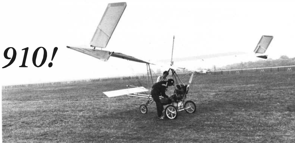
The Pterodactyl Ascender uses ruddivators, which both turn and bank the craft.
