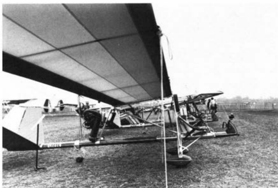
Maxair Sports' Hummer uses a single-be fuselage. Its pilot sits way out front.
