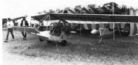
Flight Designs' Jet Wing (below) has a conventional delta wing like a hang-glider and is flown either as a hang-glider or a powered ultralight.
