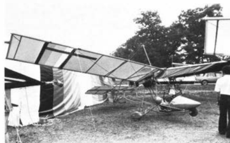
Evolved out of an unpowered hang-glider, the Quicksilver MX protects its pilot with a streamlining nose cone.
