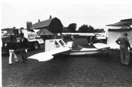
The American Eagle uses weight shift like a hang-glider instead of controls. Its wings carry ruddivators.
