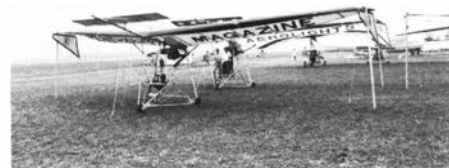
The American Eagle uses weight shift like a hang-glider instead of controls. Its wings carry ruddivators.
