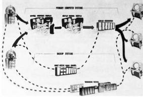
"Hot standby" is DARC's normal mode of operation. While the primary NAS is functioning, DARC parallels it, feeding digitized data through its minicomputers. Only when NAS is down is DARC switched on and its data displayed.
