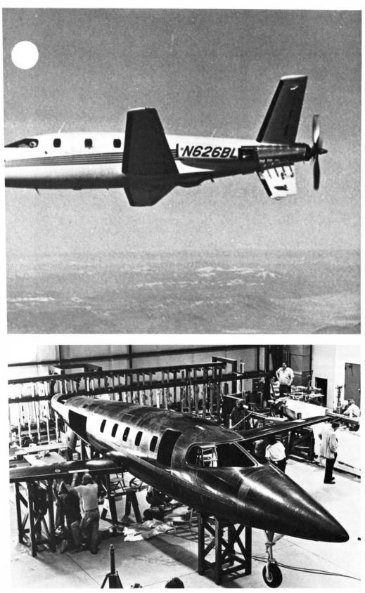
A prototype for demonstration purposes is assembled with some riveting to hold the epoxy-bond panels in place while being cured, in lieu of the tooling needed for an :poxy-only bond. For certification, the prototype will only be bonded.
