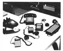
If a Touchtone push-button telephone (center rear) isn't available, a variety of tonegenerating keyboards can be coupled to a dial phone to access VRS.
