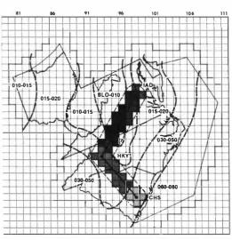
A graphic display of an ARF route-oriented briefing shows grid cells of weather for a corridor from Dulles to Hickory, N.C., to Charleston, S.C.
