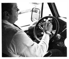
His throttle is a motorcycle-type control at his left hand; three pegs on the steering wheel support his weakened hand for spinning it.
