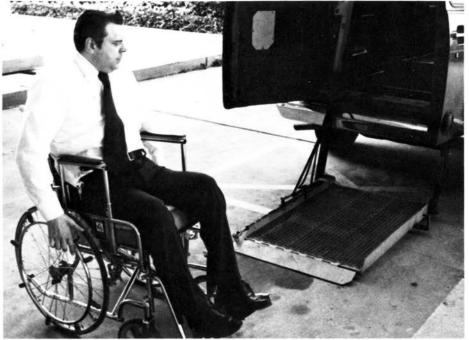
He enters the van facing forward but turns around to leave to assure himself that the platform is fully lowered. The control panel for the lift and doors is on ne left door. Because the Blue Max couldn't fit in the agency garage, a service driveway space was provided and a curb cut installed to permit Ken Hawkins to enter the building at terrace level.
