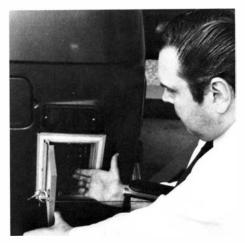
Hawkins' solo performance with the Blue Max starts with a toggle switch panel on the rear fender, which opens the doors and lowers the lift gate.
