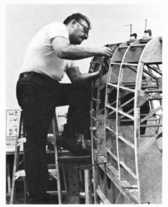
Museum technician John Cusack restores the wing of a Northrup 1NM Flying Wing, carefully regluing joints and replacing dryrot with faired in pieces of wood.
