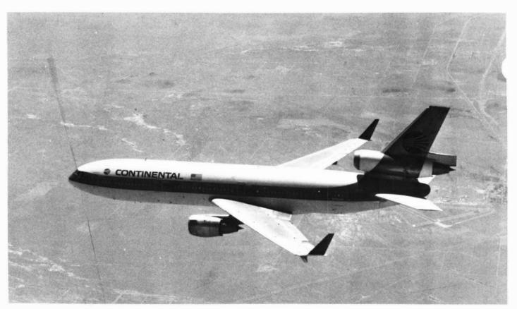
In a joint project with the National Aeronautics and Space Administration, McDonnell Douglas is testing winglets on a Continental Airlines DC-10. Projecting 101/2
