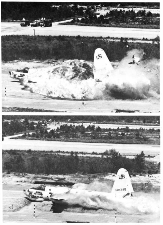
In a test at Lakehurst, N.J., when a transportcategory aircraft loaded with regular jet fuel was hurtled along a catapult into a mound of earth and fuel was spilled and ignited, the plane was engulfed in a ball of flame.
