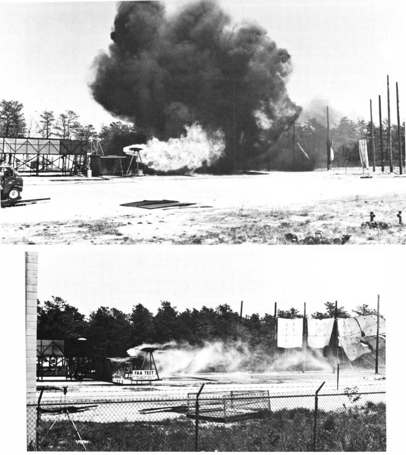
Standard aviation fuel spilled from a wing section and ignited at the FAA Technical Center's Wing Spillage Test Facility goes up in a huge fireball. (top) The same test set up for fuel with 0.3 percent of FM-9 antimisting additive is a fizzling success--no fireball. (above)
