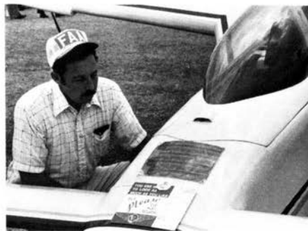
Milwaukee FSDO chief Tom Howard examines a new addition of a solar photovoltaic collector to a popular EAA show design—the Vari-Eze canard.
