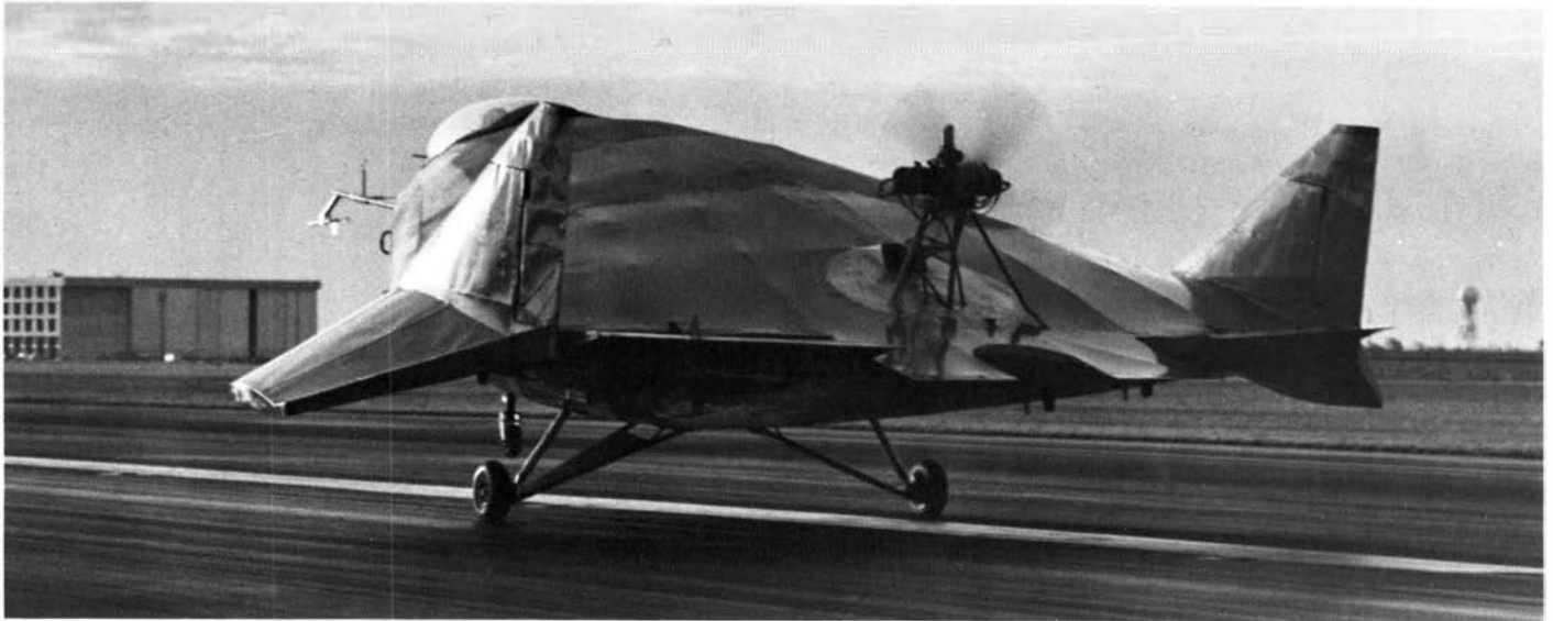
The Aereon 26—the “Deltoid Pumpkin Seed”—a lifting body that combines aerodynamic and aerostatic qualities—made six successful flights to 1,000 feet at NAFEC in 1970. With helium added, it could reach higher altitudes.
