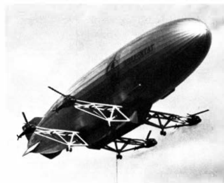
An artist's rendition of the hybrid Piasecki Heli-stat, which would combine the lifting power of a non-rigid airship with four helicopters. It's being developed under a Forest Service contract.
