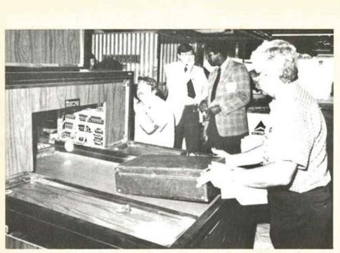
**BETTER BOMB DETECTOR**—Theo Tsacoumis of Headquarters' Civil Aviation Security Division feeds baggage into a new machine developed by DOT's Transportation Systems Center for detecting explosives. Here at Logan International Airport in Boston, project chief Dr. John Hobbs adjusts the "decompression screening system," as Bill Fogerty (left, rear) and Earl Mallard of New England Region's Air Transportation Security Field Office stand by.
