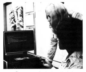
The prototype of an interim modernization now being installed at 150 busy FSSs is at the bicago FSS. It consists of a CRT display and input device, a small computer updated by the Weather Message Switching Center in Kansas City and a backroom bank of television cameras that transmits weather facsimile maps to the CRTs at specialists' positions.
