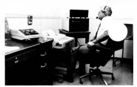
NAFEC's Dr. Donald W. Connolly has been developing a computer-operated Utterance Recognition Device (URD) that FAA hopes can be programmed to recognize human speech, thus permitting pilot briefings and filing of flight plans directly with a computer under the future FSS automated system. This would reduce the need for personal pilot briefings.
