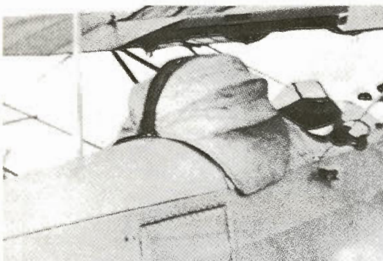
Doolittle used the sturdy Consolidated NY-2 for blind flying under a zip-up hood.
