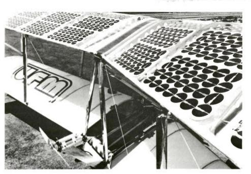
Larry Mauro demonstrated his Solar Riser-the first solar-powered aircraft-at the Experimental Aircraft Association's annual fly-in at Oshkosh, Wis., last summer. The upper wing is arrayed with 600 photovoltaic cells that power a 4-hp electric motor ... briefly. (Ultralight Flying Machines photo)
