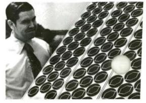
Bill Watson, assistant manager of the Kansas City International Airport Sector, looks over an array of photovoltaic cells, which charge batteries that run the ILS outer marker.
