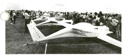
The Quickie is an unusual canard design: The wide-spreading wheel struts carry the elevators. Its 18hp engine pulls it an average 110 mph at a miserly 65 miles per gallon.
