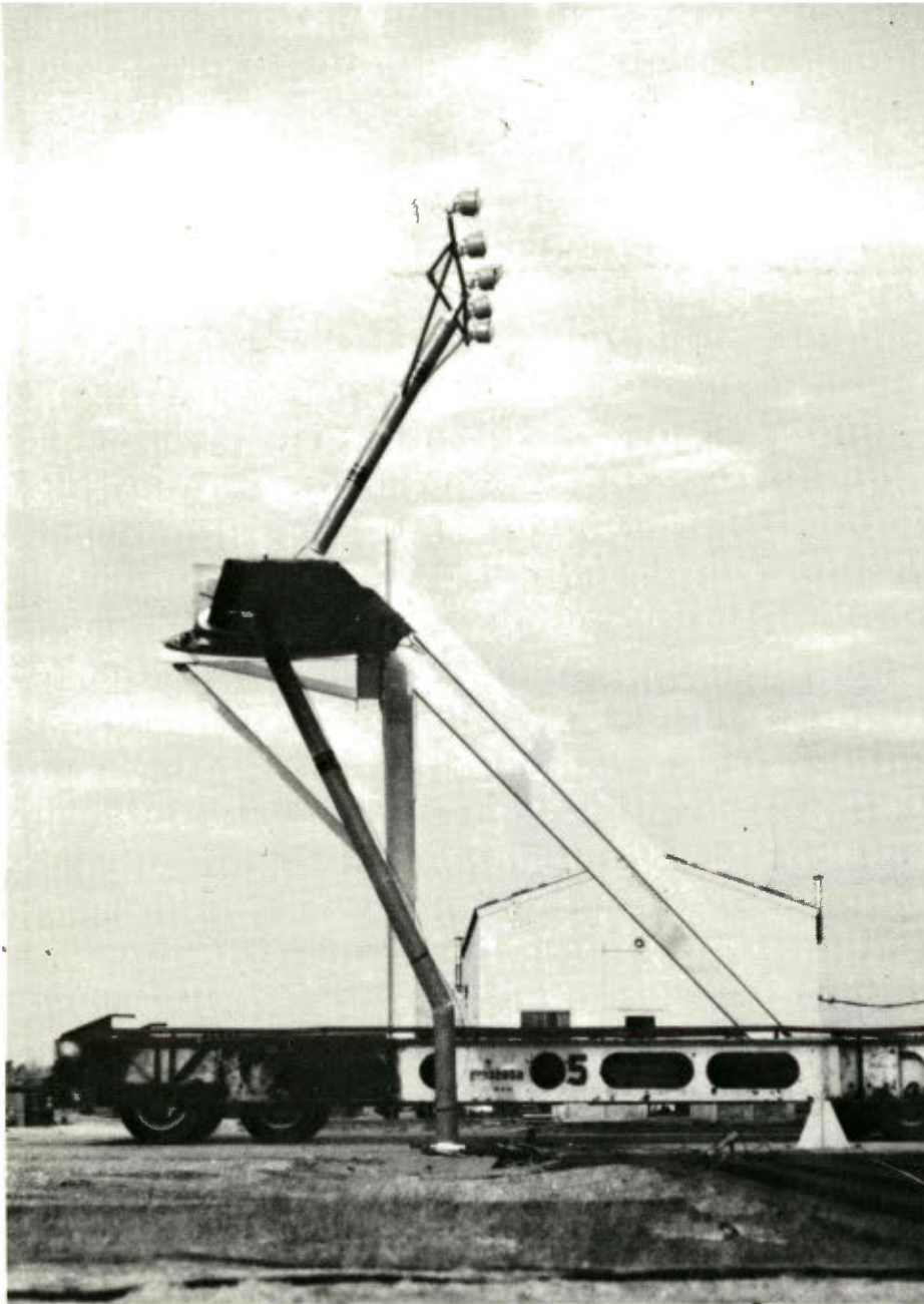
A light-aircraft wing section driven along at normal landing speed slices through a frangible fiberglass approach lighting tower in a test at the Lakehurst Naval Air Station, N.J. The breakage pattern shows the multiple fracture points, which are located every 42 inches along the shaft. The cables pull loose from a coupling at the base.
