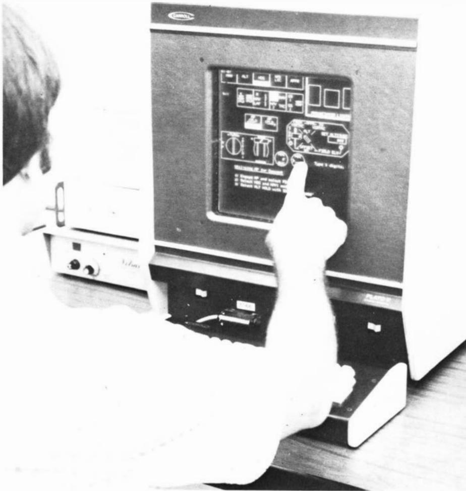
*A student punches a "button" on a touch-sensitive computer-based learning terminal, and the airborne navigation equipment depicted reacts accordingly.*
