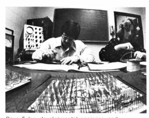
Dave Euler, developmental engineer, and Candy Dobkins, electronics technician trainee, assemble re-enforced-rate computers, which consist of integrated-circuit boards and a forest of pins and wires.
