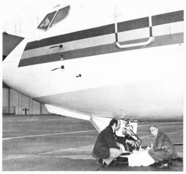
WHEEL DOCTOR—Leroy Gammon, Seattle Engineering and Manufacturing District Office inspector (right), and Bill Broadhurst, Boeing Co. engineering liaison, check over the B-737 wheel gravel-and-rock deflector that protects the belly of the airliner upon landing.
