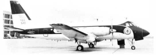
Flying in support of the center's collisic avoidance system (CAS) tests is N-48, on, of two Gulfstream 1s. It is also used for RNAV research and is equipped with avionics for CAT II flight for runway-lighting.
