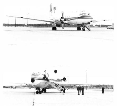
The four-engined N-42 is a Convair 880, which is configured for testing ILSs and the time-reference scanning-beam microwave landing system, and contains the most advanced flight directors and a digital autopilot. It is NAFEC's largest aircraft.
