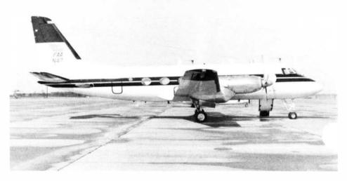
The Convair 580 turboprop—N-49—is also instrumented for use in the development of CAS and has CAT II capability for the runway-lighting programs. It also sees service for Omega and Loran-C testing.
