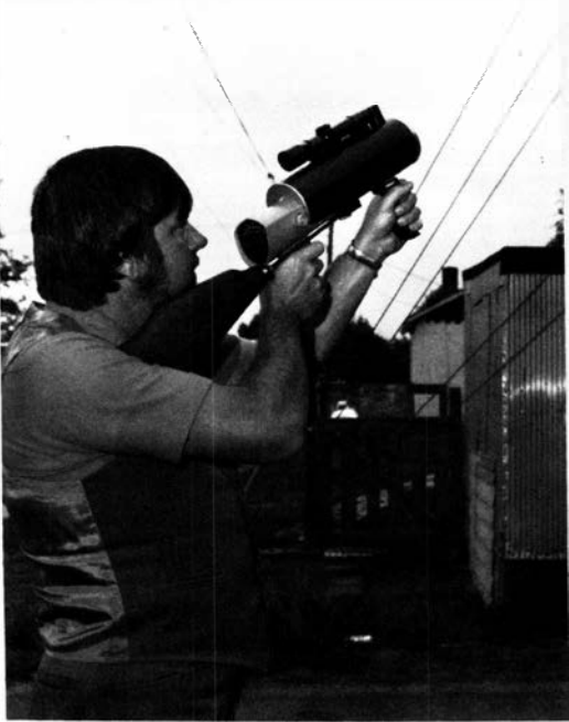
SNIPING AT PROBLEMS — Neither bazooka nor ray gun is in the hands of Edmund P. Kennedy, Rocky Mountain AF Division assistant chief. It's an infrared heat detector that can spot noise sources on overhead power lines. It can hit a two-inch target at 40 feet.
