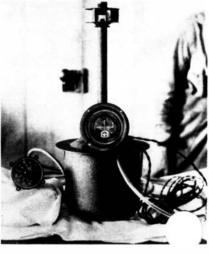
The shaft of the earth-inductor compass passed through the top of the fuselage to catch the wind; the tub holds a rotating armature; the dial at left is for setting a heading; the other dial is a left-right indicator.
