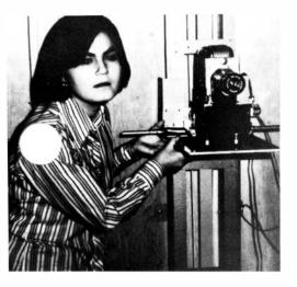
points and then feeds 40 measurements into a computer. In a minute and a half, it can measure even the squirmiest child.
