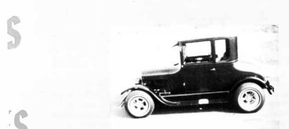
NOT JUST FOR SHOW — This rebuilt Model T coupe has won several national awards for "Best Engineered" for Allan Ashbury, air carrier operations inspector with the San Francisco ACDO. Driven daily, the car actually boasts a 289-cu. in. Ford engine with automatic transmission, power brakes, power steering, a Jaguar suspension, air conditioning, and, of course, a beautiful exterior.
