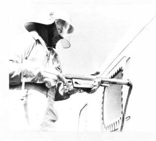
FIRE-FIGHTER—No, it's not a rebel soldier from Princess Leia's starship! It's Chuck Urban, NAFEC aerospace engineering technician, testing an aircraft-skin penetrator nozzle developed by the USAF for injecting extinguishing agents to combat fires inside aircraft.
