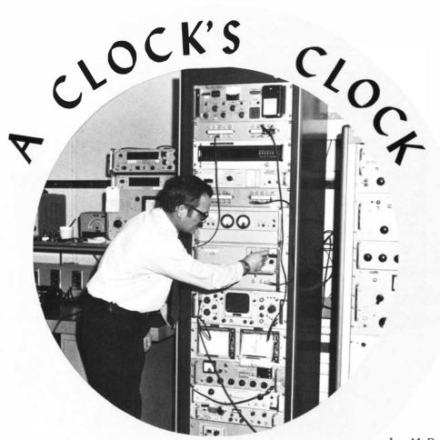
Ira McDaniel makes an adjustment on FAA's most accurate clock installed at NAFEC. The cesium-beam atomic clock is accurate within six ten-millionths of a second for time and frequency.
