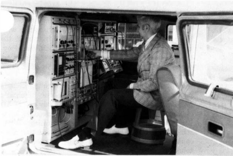
INTERFERENCE BAN VAN —Increasing congestion of radio frequencies has resulted in greater interference with aviation frequencies from such things as plastic welders, ships, garage-door openers, cars and other radio stations. To the rescue is this self-contained Electromagnetic Interference Van, which detects and measures the interference. John Guest, frequency manager of the Central Region operates the van.
